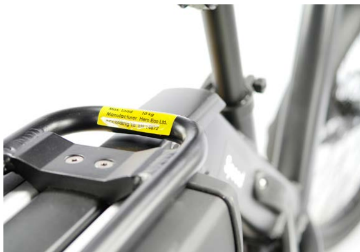
LEFT The A2B has an unconventional and very elaborate frame, distinguishing it from the bulk of other pedelecs. The battery is fitted under the carrier rack, which is limited by the manufacturer to a payload of 10 kg.
